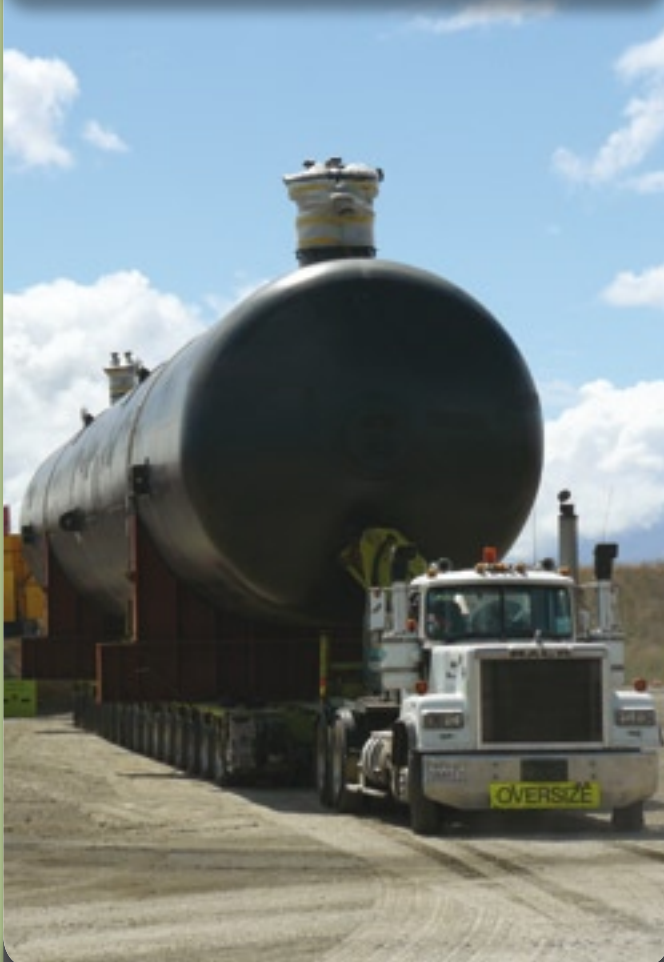
An LPG 'bullet' is delivered to the Kupe Production Station
